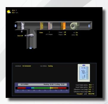
Seamless integration with the i-Vu® building automation system makes it easy to view, schedule, and manage the connected HVAC system.
